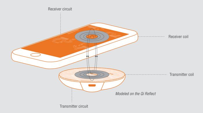
When a Qi enabled device is placed onto the charger, the transmitter in the charger will "talk" to the receiver in the device using a magnetic field.
